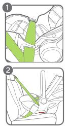
Place carrier on an approved vehicle seat location. Carry handle MUST be in position A. See page 17.
