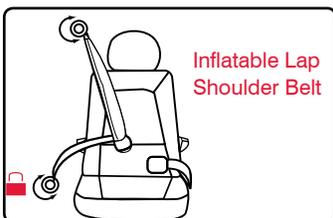
**NOTE:** To use a child seat with this type of vehicle belt, you will need to switch the retractor for the lap section of the seat belt to the ALR mode.
