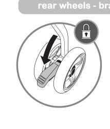
press button down to lock brake
