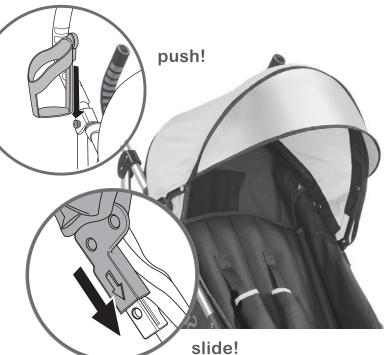
slide canopy onto frame mounts and attach velcro (both sides) 3
