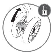
press button up to unlock brake
